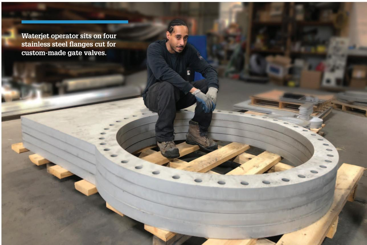
Waterjet operator sits on four stainless steel flanges cut for custom-made gate valves.
