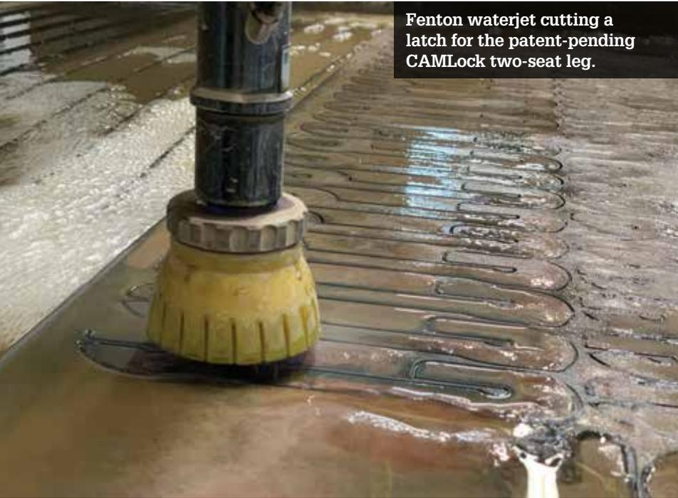
Fenton waterjet cutting a latch for the patent-pending CAMLock two-seat leg.
