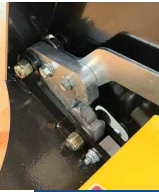
Step-N-Lock large and small latches installed in a seat base in the “unlocked” position to demonstrate an actual installation.
