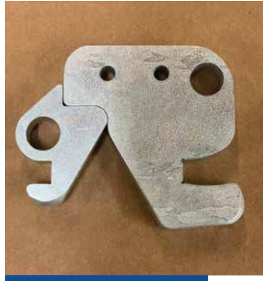
Step-N-Lock large and small latches out of a seat base in the “locked” position to demonstrate quality of fit.
