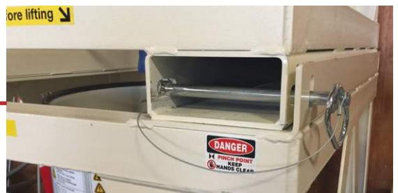
The garnet abrasive transfer hopper eliminates the time and fatigue of handling 55-lb. bags of garnet. Right: Connecting pins help hold the hopper in the stand even when bumped.
