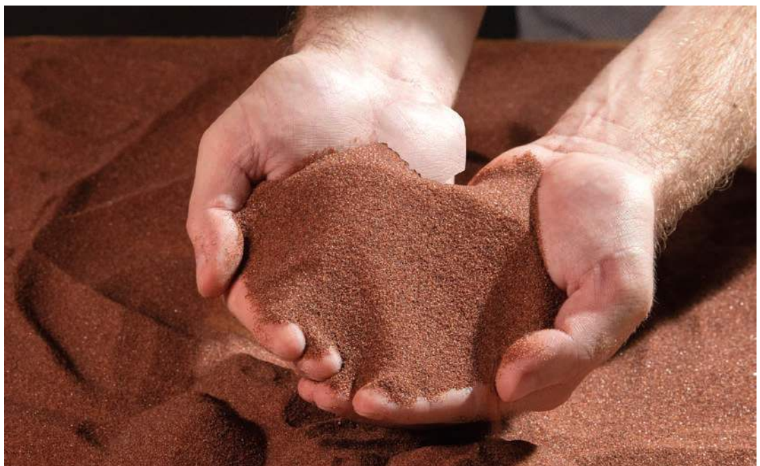
This is what garnet abrasive looks like before it enters the waterjet stream. Barton International
