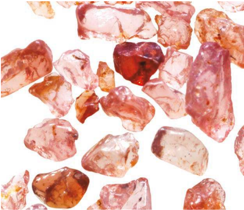
The up-close view reveals the alluvial nature of the garnet abrasive. Barton International
