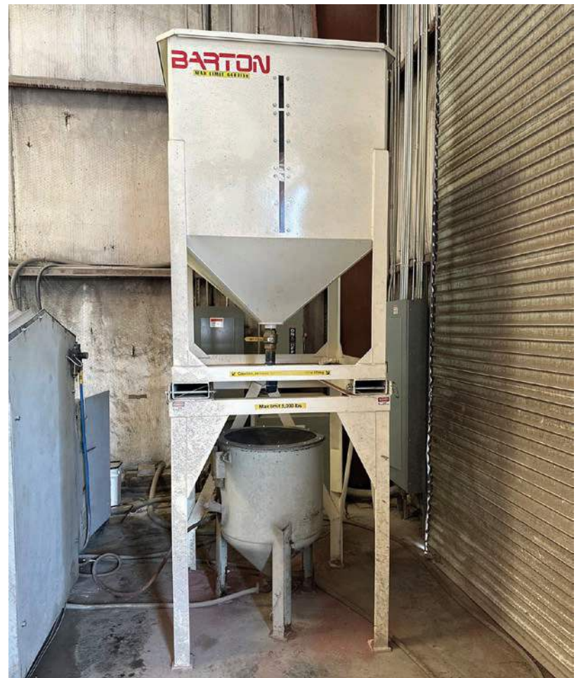
For continuous operation of a waterjet, a metal fabricator might rely on an abrasive transfer hopper, which is positioned above the pressure pot and near the waterjet cutting machine. Barton International
